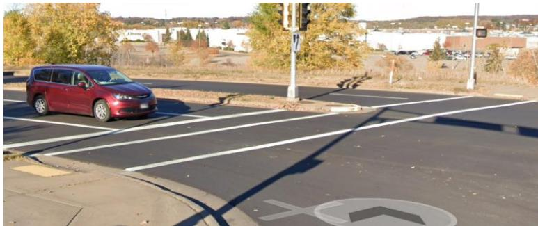
We have received complaints about the ladder-style crosswalks being slippery when wet or snow covered. Additionally, ladder-style crosswalks are time and material consuming to repaint every year.
